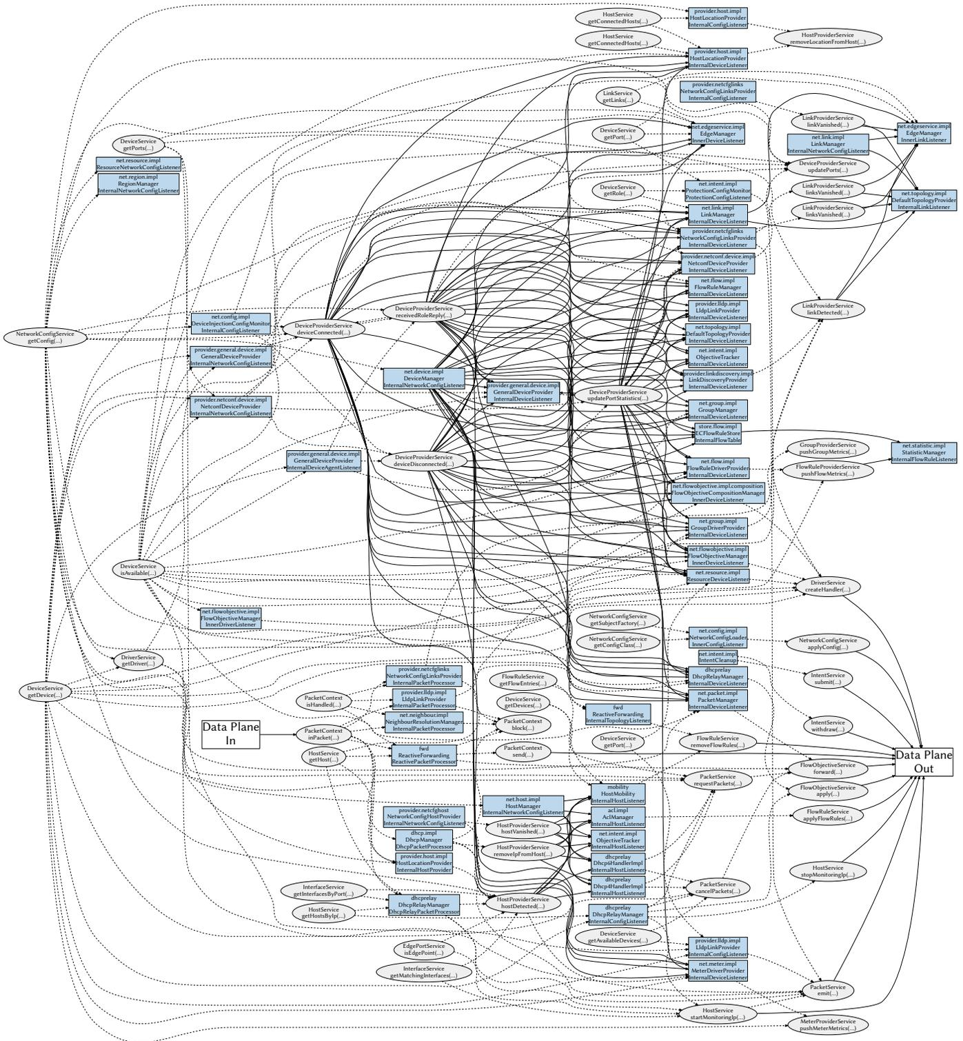
Fig. 11: Event flow graph of ONOS with core service components and several apps (*i.e.*, acl, fwd, mobility, dhcp, and dhcprelay). Blue rectangles represent event listeners and packet processors, gray ellipses represent API methods, bold edges represent event dispatches, and dashed edges represent API calls. (For simplicity, event types are reduced to a single edge of the event type's respective event kind.)
