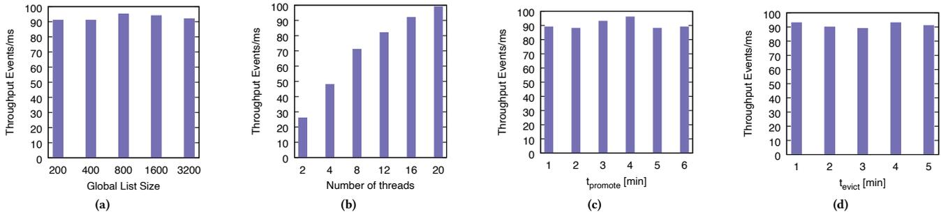
Figure 9: Throughput of SWIFT under different configuration values.
